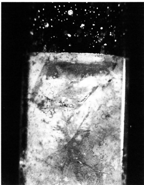
Fig. 2. \text{Li}_2\text{SO}_4 cooled below the solid-solid phase transition and then reheated to 600^\circ\text{C} .
